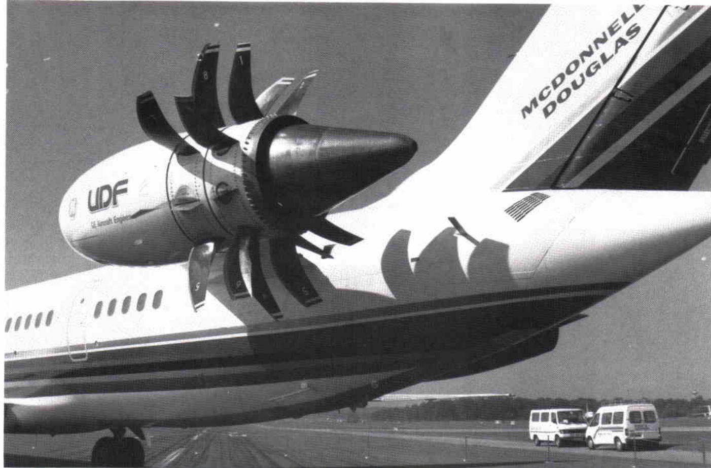
General Electric propellermotor UDF (Unducted Fan).
